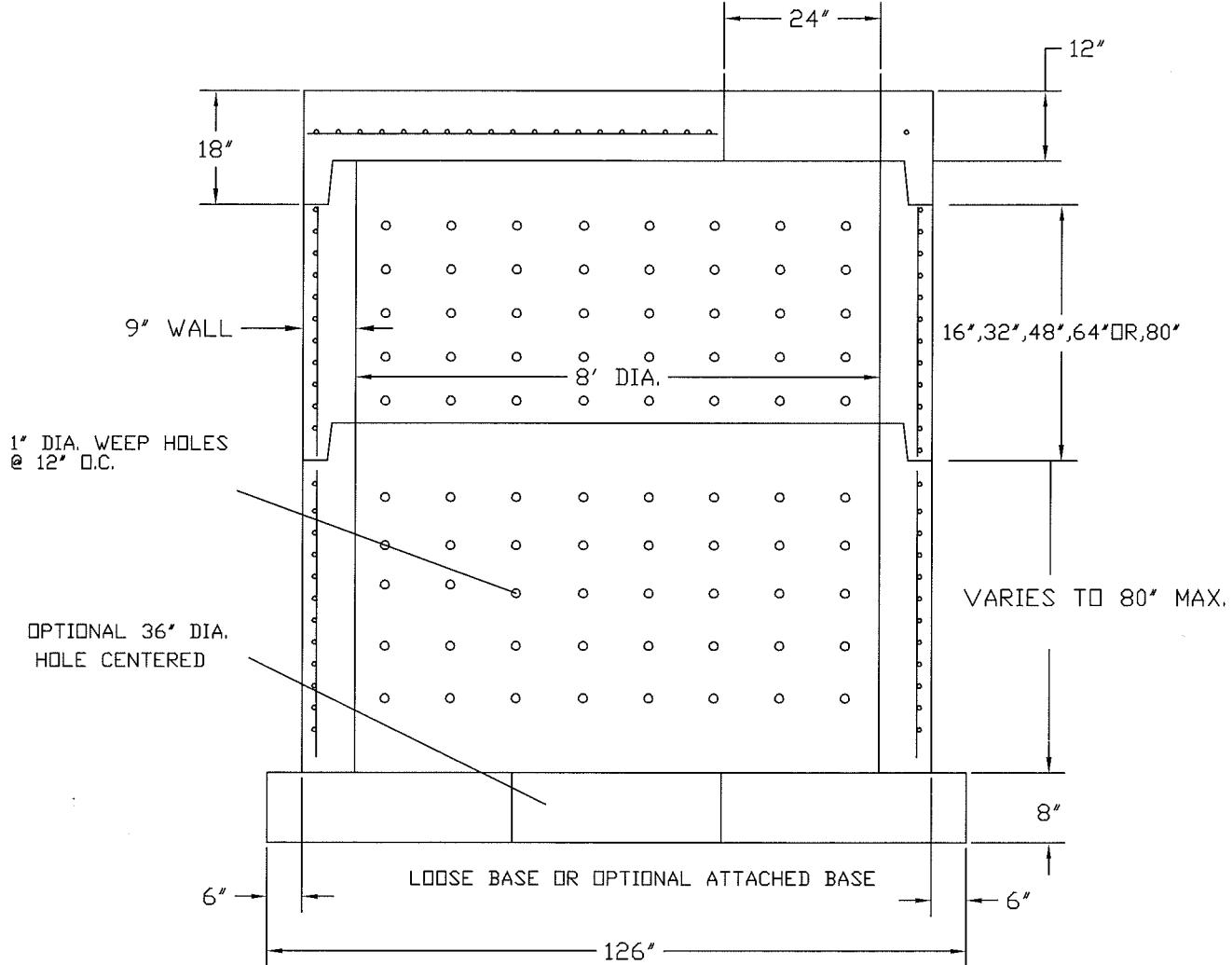
CONFORMS TO ASTM C-478
